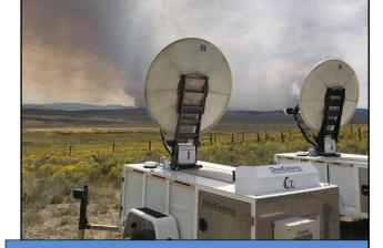
The Mini Base Camp Trailer is a deployable cell tower when NO cellular services are available. It generates an area of FirstNet (Band14), Verizon, AT&T, and T-Mobile Cellular with Wi-Fi coverage.
